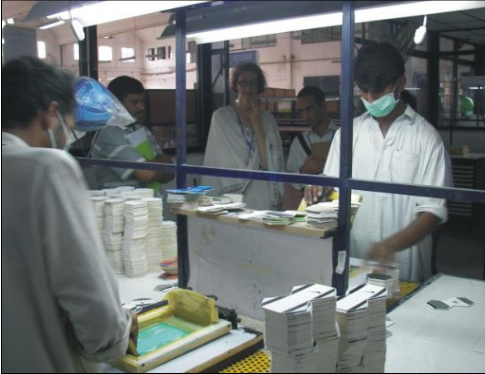
Figure 4: Screen-printing of PU panels at Silver Star's factory, September 2007
